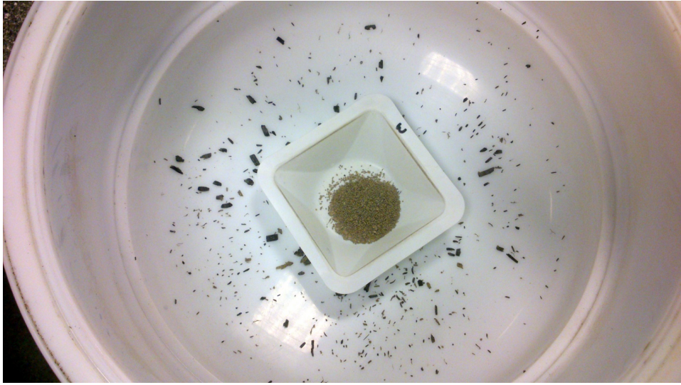
Fig. S5. In-house method for separating heavier soil particles from lighter biochar particles, whereby air is blown gently on to the soil sample (in the plastic dish) to expel biochar into the surrounding bowl.
