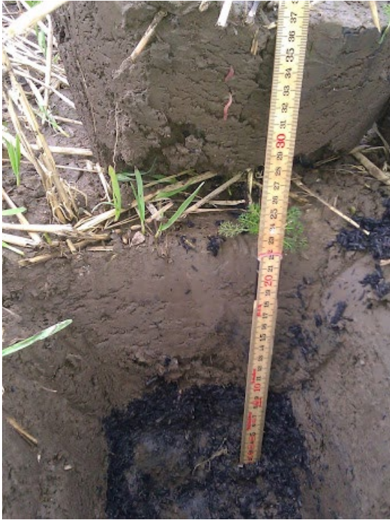
Fig. S6. High Biochar concentrations located at bottom of the plough layer (23 cm depth) in October 2011 due to ploughing in of surface applied biochar at the start of the experiment in October 2010.
