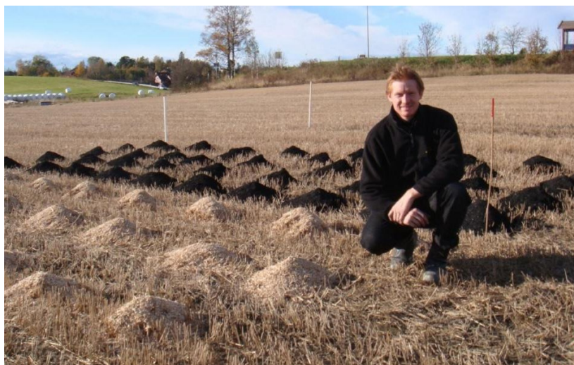
Fig. 5 Miscanthus biochar and Miscanthus chipped straw was dosed out according to its C content to allow for comparison of C mineralization rates
