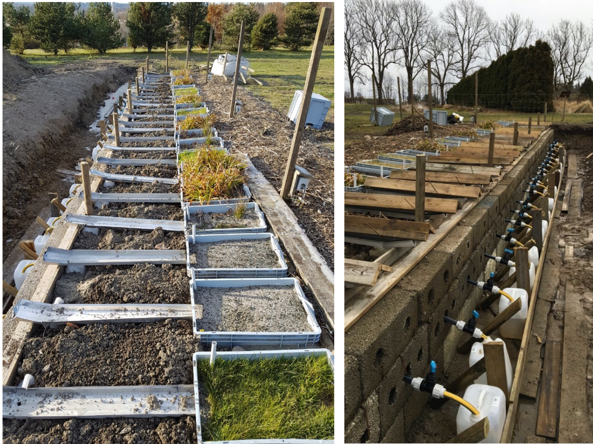
Figure 1.10 Mesocosm set up at Planteskolen, NMBU. Right picture show top of plant boxes and surface runoff system left picture shows system for collection of drained water. (right pic. Marina Bakhtina 5. Nov 19)
