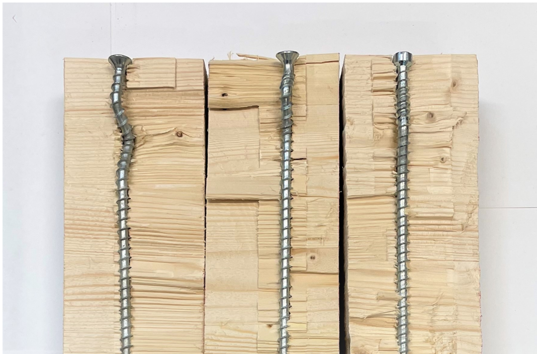
Figure 6.6: Failure HT-T 8.0x300, 8.0x340 and VGZ 9.0x440
