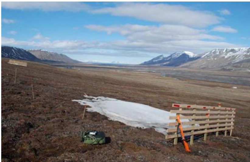
Figure 3 : Photo (©Elizabeth Cooper, (Cooper, Dullinger, & Semenchuk, 2011)). Photo of snow fences at Adventdalen in Svalbard
