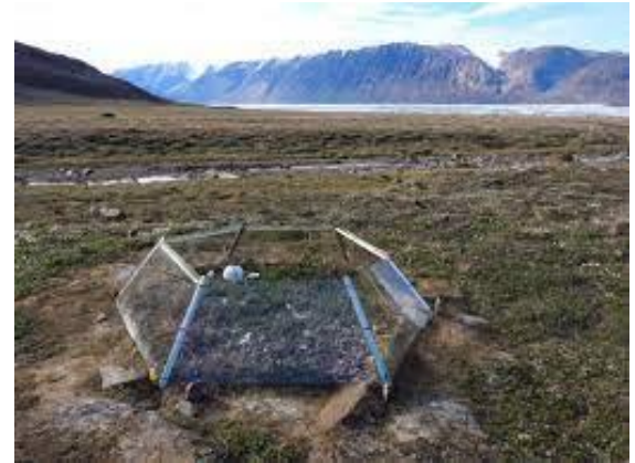
Figure 4: Photo (©Cassandra Elphinstone, (Elphinstone, 2018)). Illustrating open-top chamber (OTC), at Alexandra fiord on Ellesmere island in 2018.
