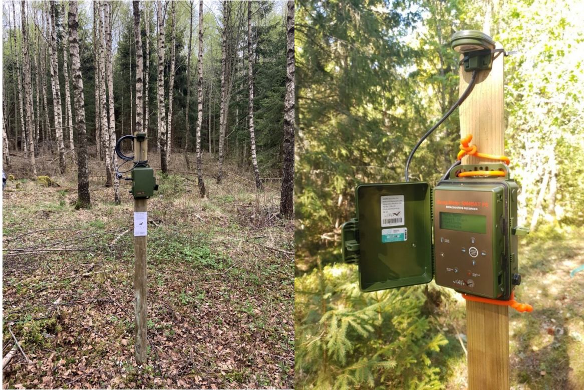
Figure 3. Setup of SM4-BATFS acoustic bat detector deployed with a U2 microphone at an open forest site.
