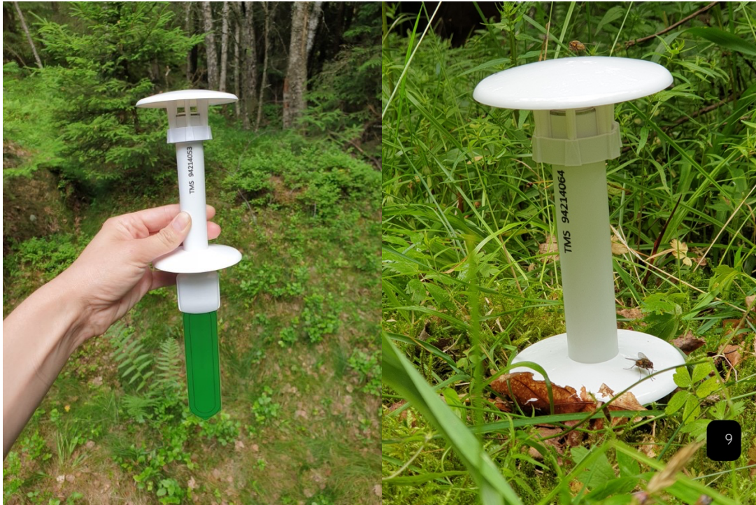
Figure 7. TOMST TSM4 soil moisture and temperature data logger before (left) and after (right) deployment with the specific serial number.
