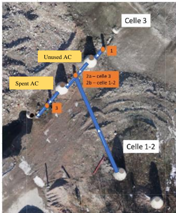
Figure 7: An overview over the sampling site. Cell 1-2 containing PFAS contaminated masses from airports and military bases, Cell 3 containing PFAS contaminated masses from drill cuttings. The blue line indicates the pipes from the cell to the wells, white arrows show the direction of the water flow. First well containing unused/new AC, second well containing used AC. 1, 2a, 2b and 3 indicates different sampling sites.
