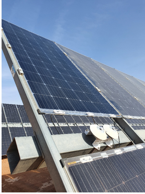
Figure 2.8: A soiling measurement station in one of the plants in this thesis. This particular station consists of two panels mounted in an array with other panels.
