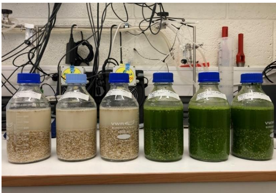
Figure 8: Control and 20% microalgal biomass substitution brewing trials, performed in triplicate in 0.8 L volumes
