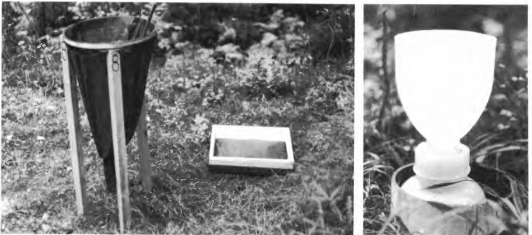
Fig. 5. The throughfall and the litterfall collectors
