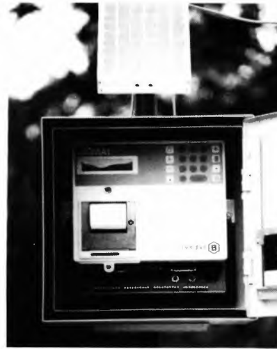
Figure 1. Solar-powered BIOMAT for field use
