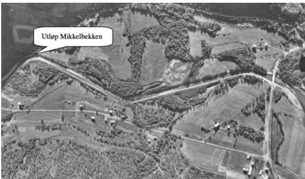
Figure 3. The lower part of Bognelv in 1972. The river has been channelized and streamlined and the natural erosion and sedimentation processes were lost (Hoseth & Josefsen, 2005).
