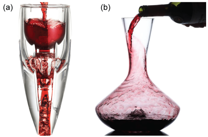
FIG. 3 Wine aeration. (a) Oxygen injection using the Venturi effect: The wine moves down into a narrow funnel by gravity. In the funnel the liquid accelerates, which lowers the pressure compared to the surrounding atmosphere, as described by the Bernoulli principle [Eq. (6)]. Hence, air bubbles are drawn in, which aerate the wine. (b) Wine decanter: By pouring and swirling the liquid around, ripples form that mix in oxygen efficiently. Images from Vintorio Wine Accessories, with permission.
