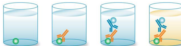
Figure 15. Illustration of indirect ELISA. Immobilised antigen at the bottom of the wells is recognised by an unlabelled primary antibody, which is in turn detected by a secondary enzyme-linked antibody [72].
