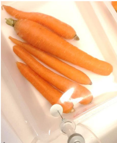
Figure 7. Measurement of gas concentration in the headspace of the packages. The gas analyser measures the gas concentration with the help of a needle connected to the gas analyser, through a septum placed on the top film. Photo: (Torstein Kvamme, 26.02.21)
