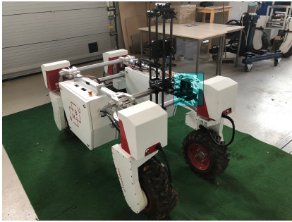
(a) Agricultural robot Thorvald with a 2D LiDAR sensor
