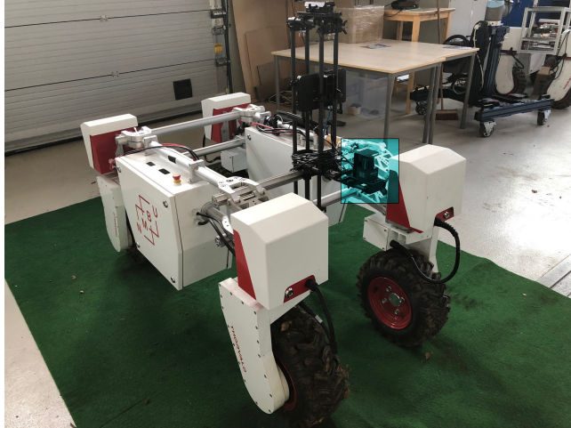
Figure III.13: Robot setup, a 2D Hokuyo laser scanner UST-20 LX is mounted in front of the robot as shown in the highlight area.
