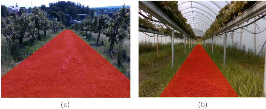
Figure IV.6: Screenshots of annotated images for training, where red areas depict traversable areas.
