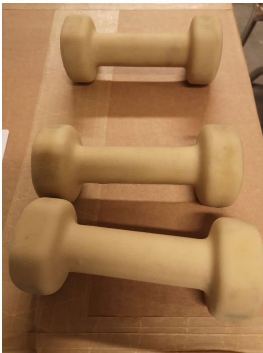
Figure 10. 1 kg dumbbells were added in the cement mixer together with Asparagopsis taxiformis .
