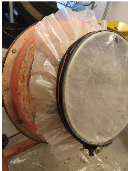
Figure 11. The cement mixer sealed with a plastic tarp, fitted rubber tube, and loading strap.
