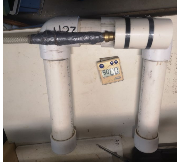
Figure 13. Gas collection yoke being prepared for gas sampling.
