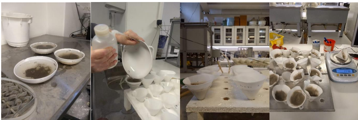
Figure 2.17 – Soil left to precipitate for 6mins in ceramic bowls. Photo: Thomas Brown (2021).
