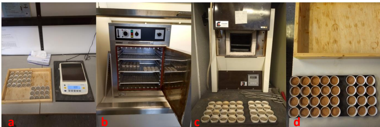
Figure 2.6 – (a) Weighing of individual crucibles with soil before (b) placing them in a drying cabinet overnight at 105 °C. (c) Crucibles containing the dried soil are placed in the calcination furnace for 3 hours at 550 °C. (d) Soil after calcination. Photos: Thomas J. Brown (2021).
