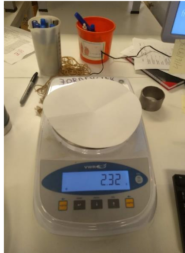
Figure 2.12 – Weighing of filter paper. Photo: Thomas J. Brown (2021).
