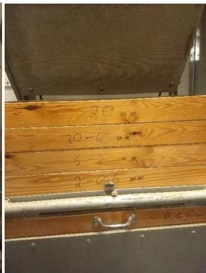
Figure 2.9 – Motorized sieve. Photo: Thomas J. Brown (2021).
