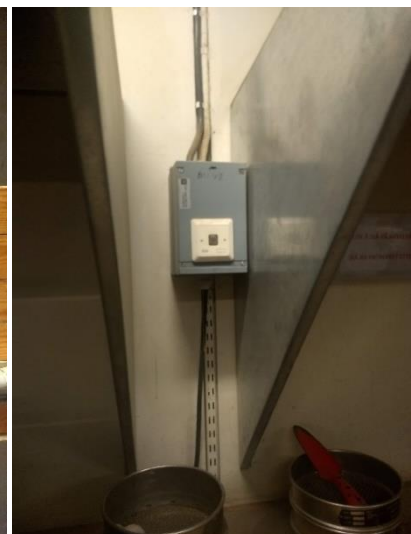
Figure 2.10 – Start button motorized sieve. Photo: Thomas J. Brown (2021).
