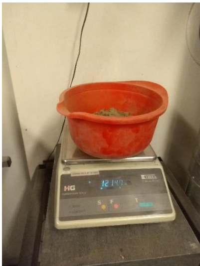
Figure 2.8 – Weighing of soil sample. Photo: Thomas J. Brown (2021).
