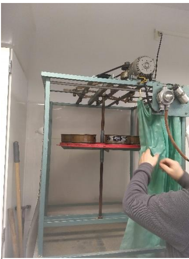
Figure 2.15 – The rainfall simulator with 4 sieves placed on the rotating platform. Photo: Thomas J. Brown (2021).
