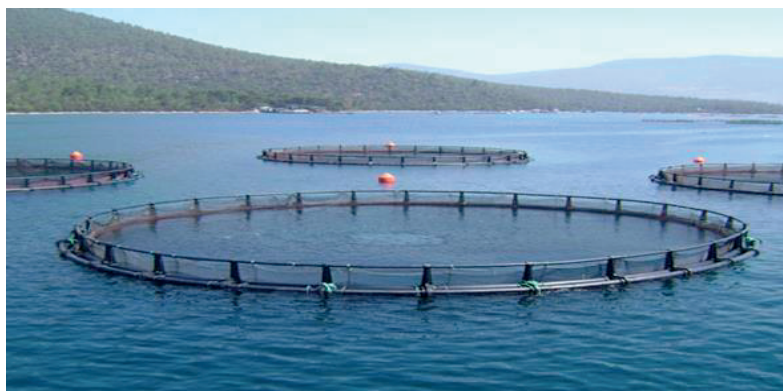
Figure 6. HDPE cages (source: http://www.tradekey.com/product-free/Hdpe-Cage-For-Fish-Farms-736231.html )
