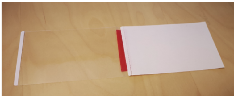
Picture 1: The plastic film as it should look when exposing. Keep the tape end connected to the protective film so that it will be easier to put the protective film back on the exposed film.
