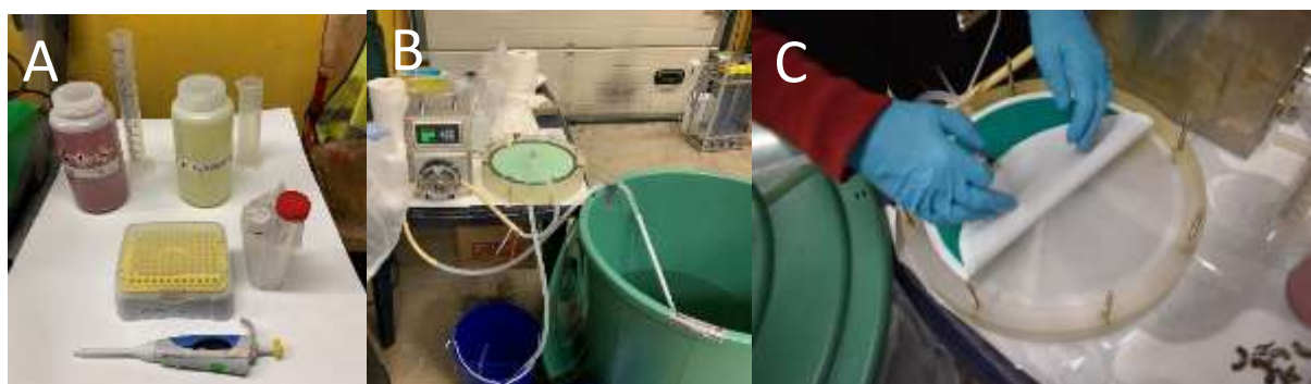
Figure 3.4: Radiochemical separation of the water samples performed “in situ” at a local workshop. Adding yield monitor, k -hexacyanoferrate, and cobalt chloride (A), pumping water through 0.45 µm filter (B), and folding filter with precipitate containing Cs-137 and Cs-134 (C)
