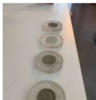
Figure 3.10: Sample holders containing freeze dried sediments, for XRD analysis.
