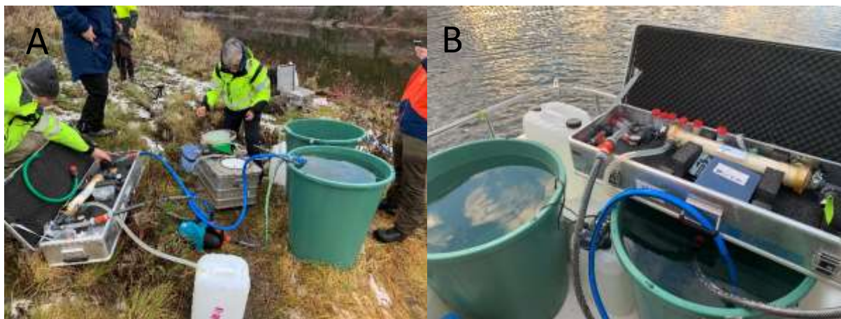
Figure 3.3: In situ fractionation of water with hollowfibre ultrafiltration and 0.45 µm particle filtration at site FW1 (A) and SW3 (B).
