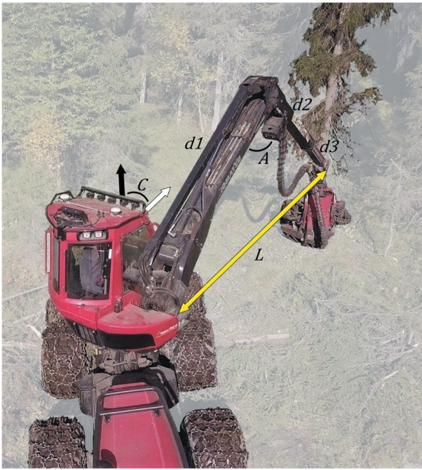
Figure 2. The Komatsu 931XC harvester used in this study, and the industry standard system for positioning harvested stems. The black arrow indicates the machine's bearing, the white arrow indicates the direction of the crane, C indicates the crane angle with respect to the machine bearing, A indicates the angle between the inner and outer boom, d1 , d2 and d3 indicate the inner and outer boom and telescopic extension, respectively, and L indicates the crane length, as calculated by the on-board computer.
