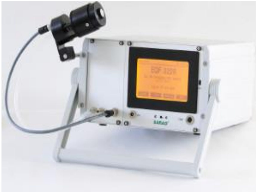
Figure 8. The new SARAD instrument is used for indoor radon concentration (SARAD n.d).
