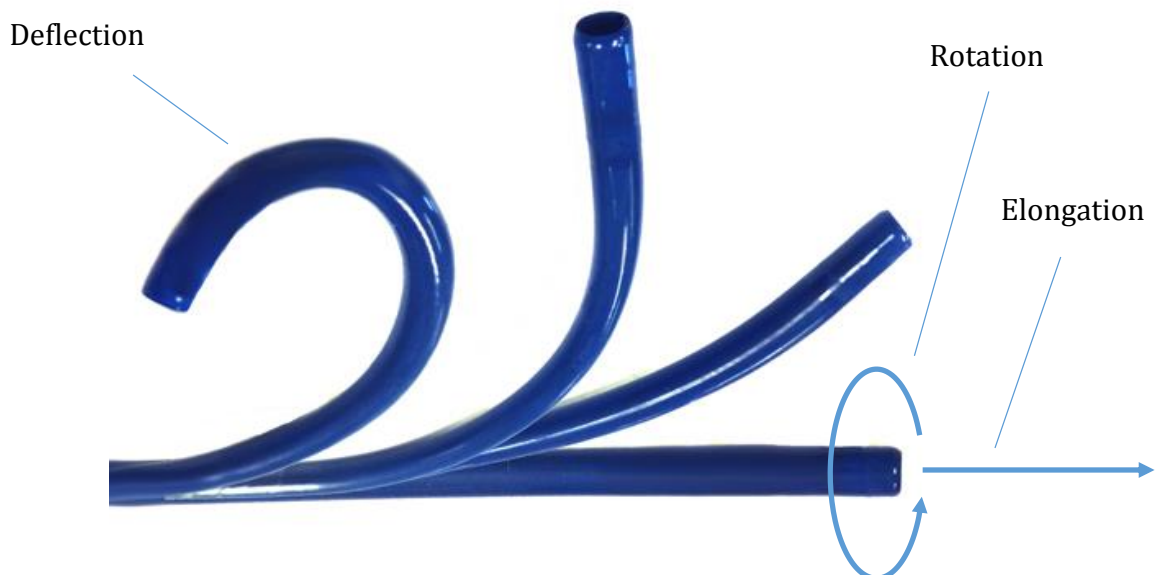
Figure 31: Illustration of deflection, rotation and elongation [39].
