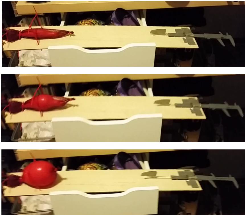
Figure 3: Three steps from when the balloon is expanding and shortened in the longitudinal direction to apply a force to the rod that its connected to. A caliper is connected to it to measure the shortened length.
