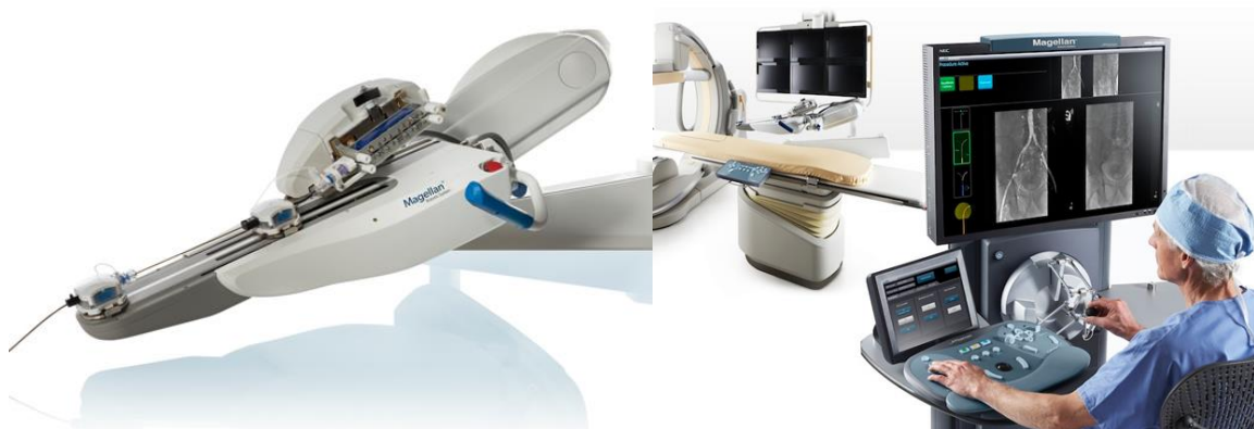
Figure 11: a) Magellan robotic system by Hansen [9], b) the surgeon remotely controls the catheter [10].
