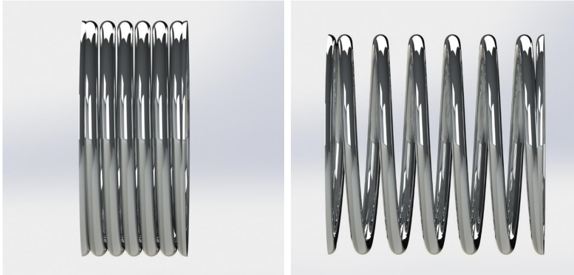
Figure 57: a) the coil spring compressed and b) the coil spring elongated.
