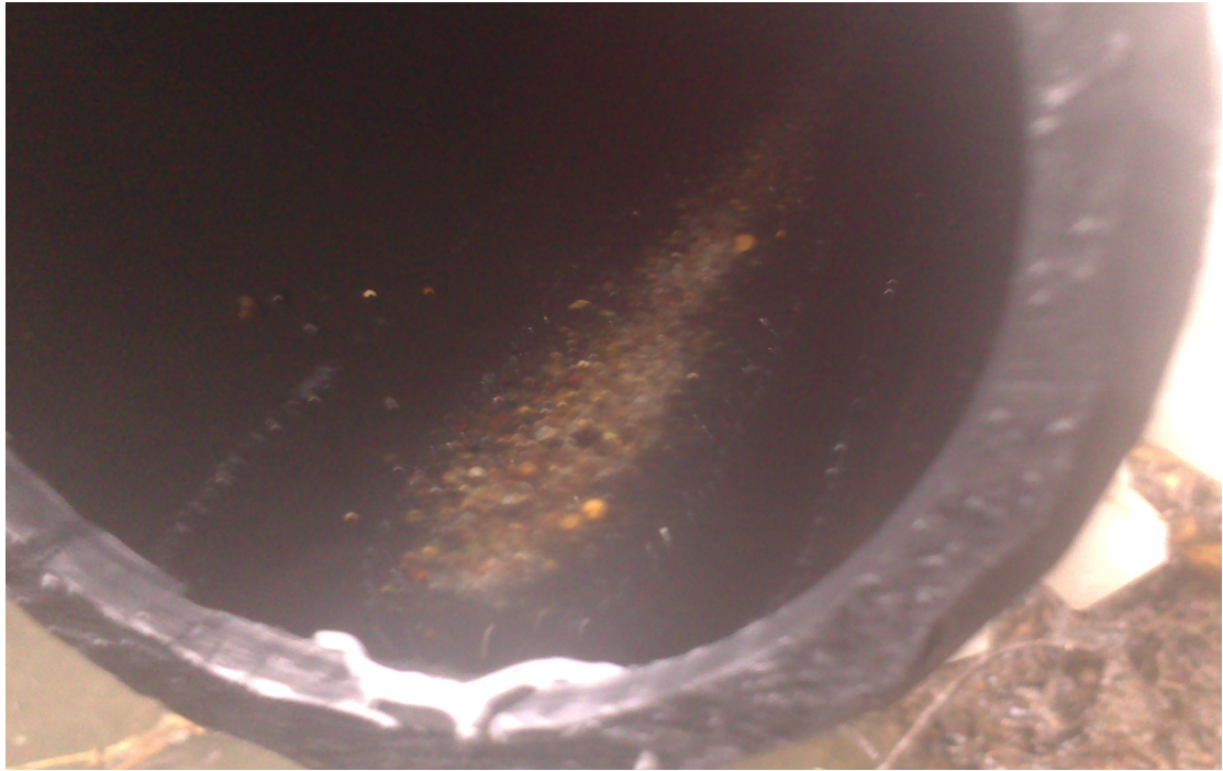
Figure 13.5: Distribution of sediments in SDR11 PE 63 mm pipe (Source: the author)
