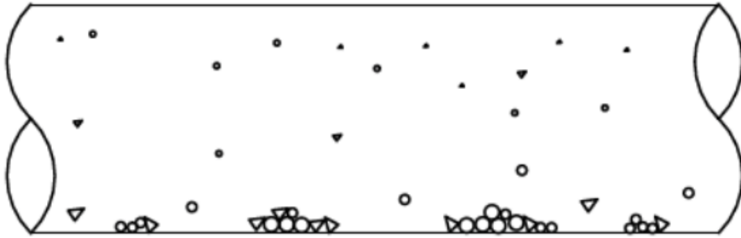
Figure 10.4: Sliding bed conditions (Copeland, 2013)
