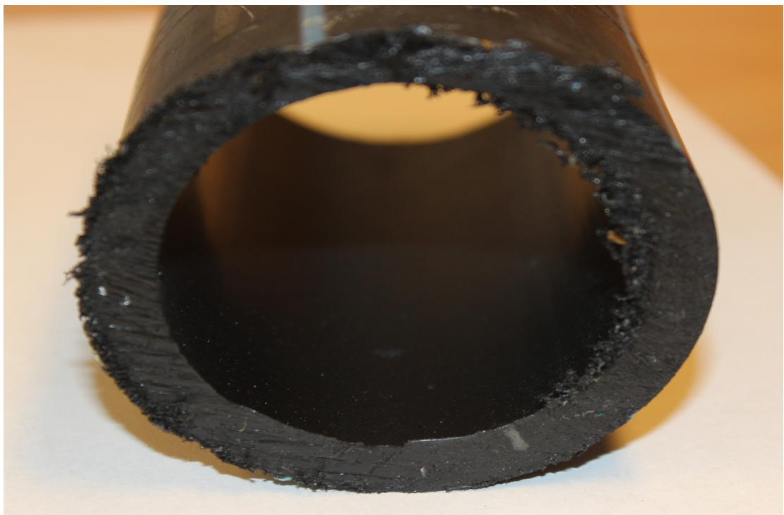
Figure 13.6: Cut off section of the SDR11 PE 50 mm pipe (Source: the author)
