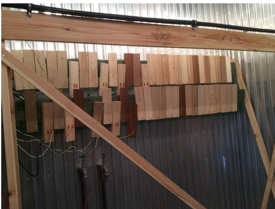
Figure 10 Climate chamber with wood samples. Wood samples with wires logged moisture. Samples were rotated every week.
