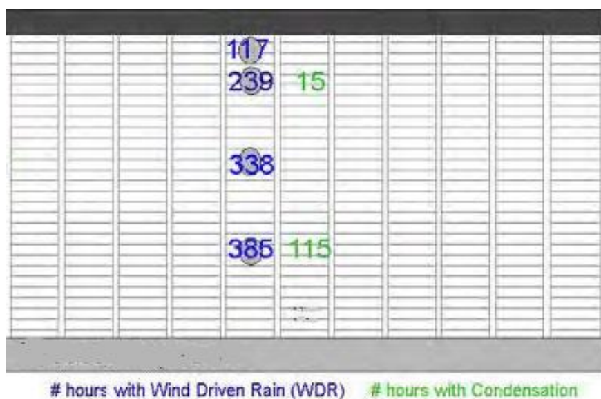
Figure 5 Wooden facade with variation in calculated hours of condensation and accumulated wind driven rain. Less condensation near the roof overhang due to less radiation loss. Adapted from Nore, 2009.
