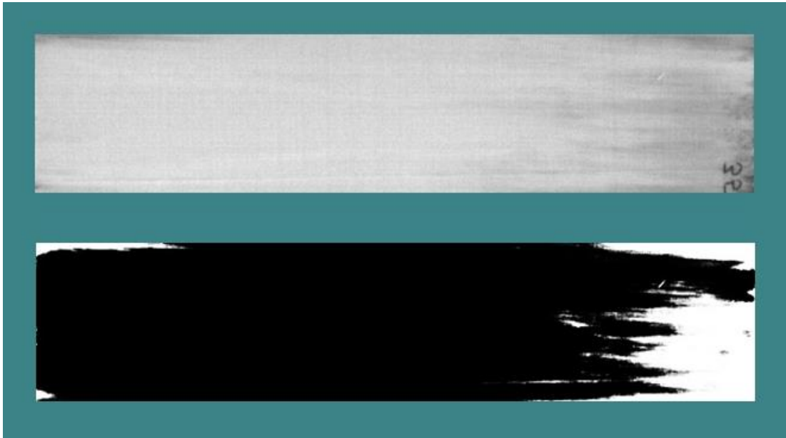
Figure 11 Hyperspectral image in greyscale on top, after PLS-DA processing showing mould white and wood black, bottom. Sample 35 after 7 weeks was estimated with Fiji to have 13% mould coverage.
