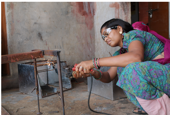
Picture 1: Constructing solar cookers 1 Source: Linn-Cathrin Juell, 2014
