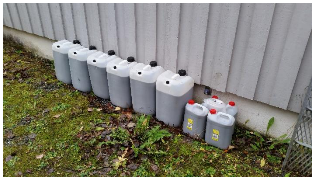
Figure 10: 25- and 5liter polypropylene water containers filled with drilling fluid (Photo: Lene Sørli Heier 2014).
