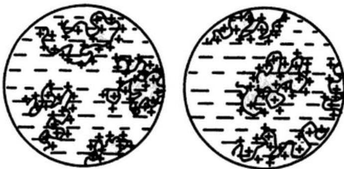
Figure 3: The "Patch theory" concept. The figure illustrates two negatively charged particles, on which cationic polymers is adsorbed unevenly (Gregory 1978)
