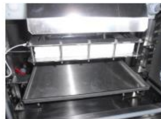
Water filled UVB or UVC filter between the water cooled flash lamp module and the sample shelf.
