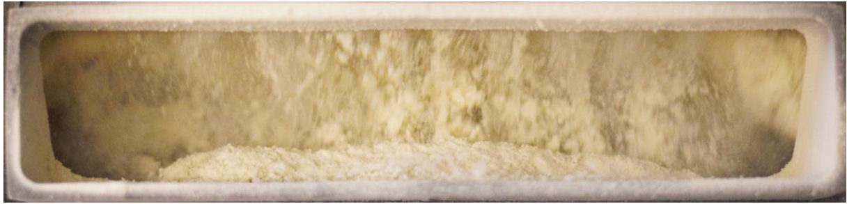
Figure 5.2: Suspended flour particle stream traveling out of the pin mill located above the picture hitting the opposite wall.
