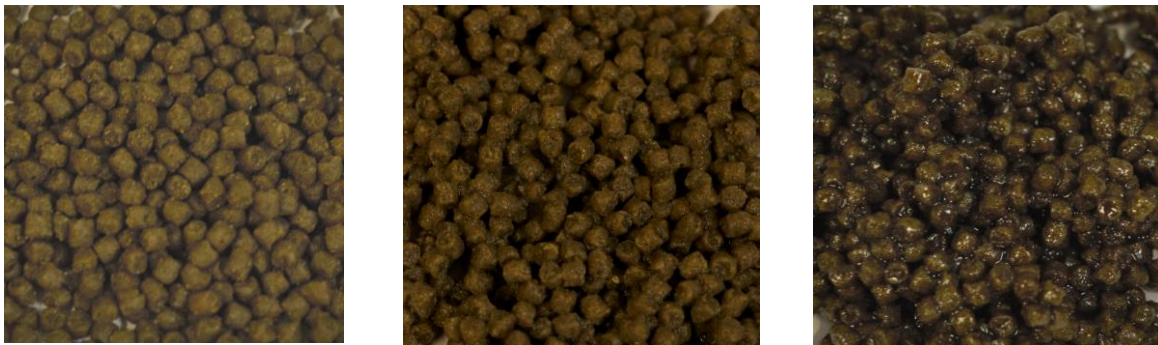
Figure 4.14: From left to right: dry pellets, vacuum coated pellets, and top coated pellets.
