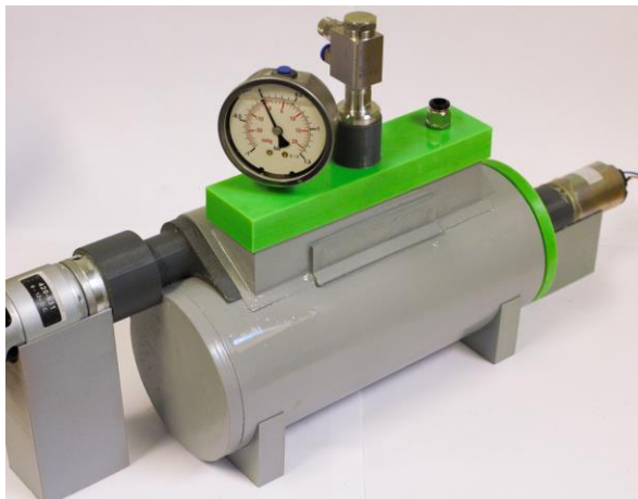
Figure 3.9: Pin mill inserted into the pin mill housing.
