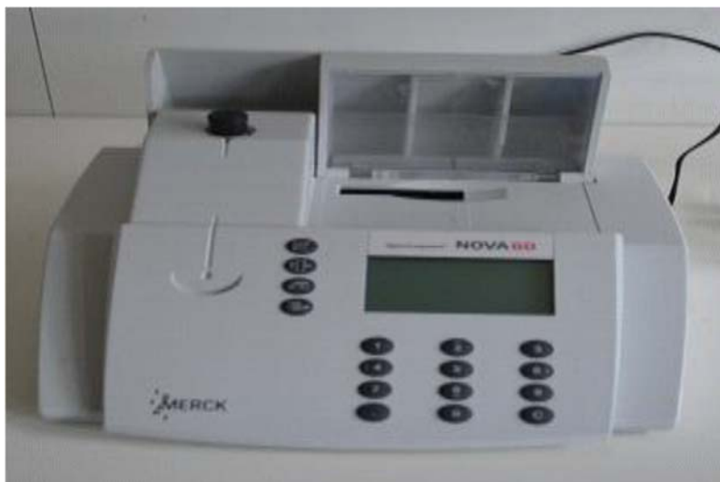
Figure 4.4 Schematic diagram of Spectroquant® Photometer NOVA 60.
