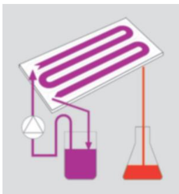
Figure 8. Setup ultrafiltration. Figure is adapted from (Sartorius 2000). The purple bottle contains the broth at which the protein was located. Both the tube entering the cassette and the retentate tubing was placed here. The last tube exiting the cassette was the waste flowing through the membrane. This was collected in the red bottle.
