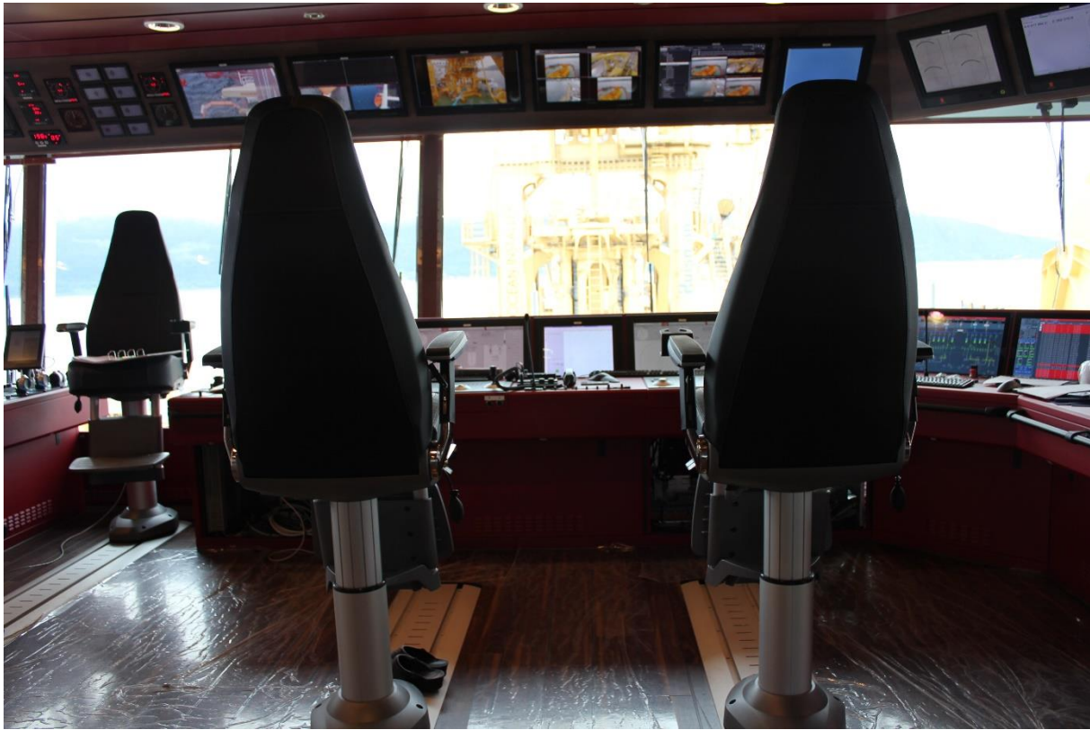
Figure 31: Aft bridge of OSCV. Workstation for ship handling is located to the left and workstation for aft support to the right. [3, 4]
