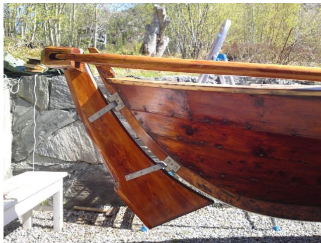
Figure 3: Hinged sternpost rudder with tiller. [9]
