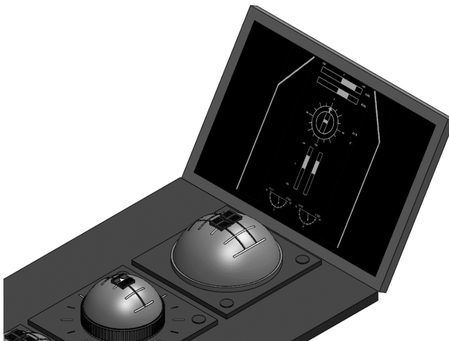
Figure 75: Close- up of azimuth lever, tunnel thruster lever and display.
