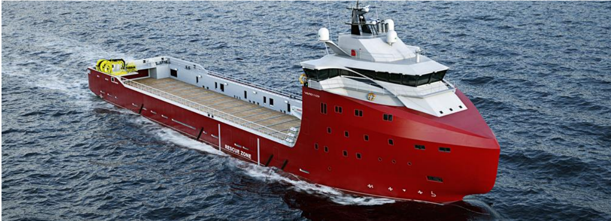
Figure 22: Platform Supply Vessel (PSV). [48]
