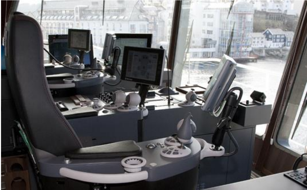
Figure 35: The Helicon X3 installed on the aft bridge DP chair. Also displayed is the Poscon DP solution. [48]
