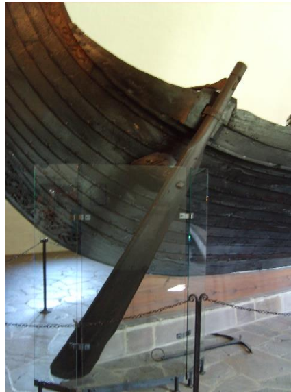
Figure 2: The Oseberg Ship, built around year 820 AD. A steering oar is located on the aft starboard side. A small tiller is mounted for easier maneuvering. [5, 6]
