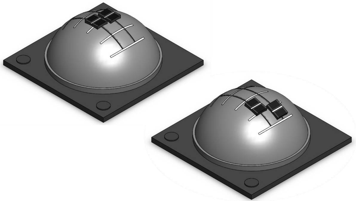
Figure 69: Left: Speed lever in neutral, forward- aft position. Right: Speed lever with approximate power on actuators of 65 % port and 30 % starboard.
