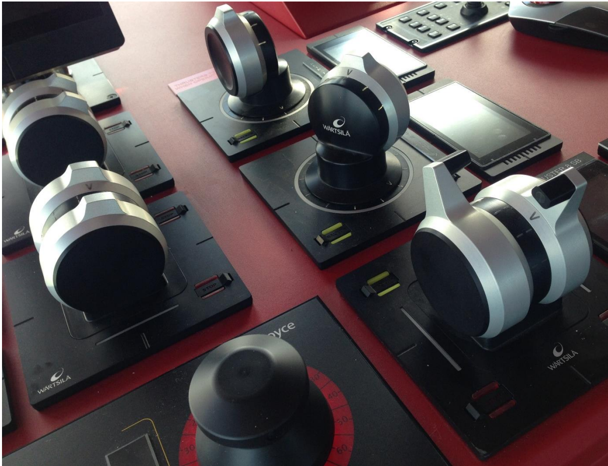
Figure 33: A typical setup of control levers. To the left two tunnel thruster levers, lower center a rudder controller (plus one out of sight), to the right a main propulsion lever and in front of it, two azimuth levers. displays are located to the right of the levers. [3, 4]
