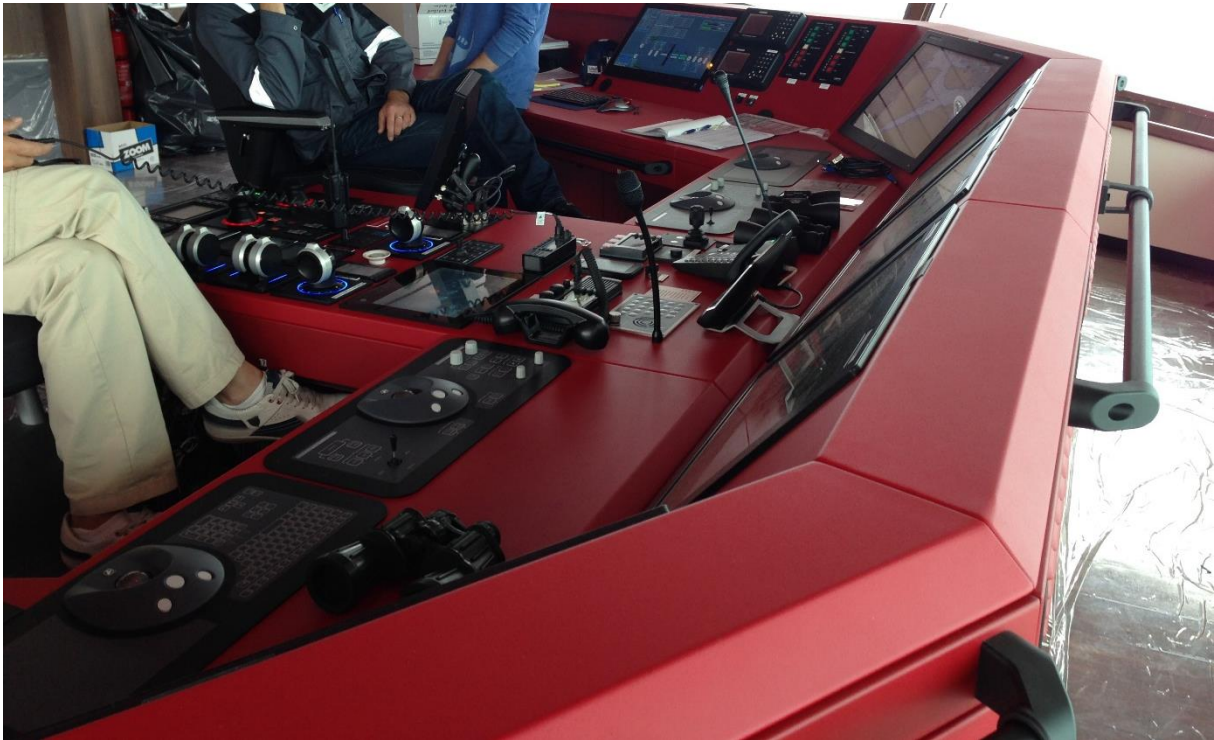
Figure 1: Typical Vard bridge. Wärtsilä control levers located center left with blue light indications on the panel. [3, 4]
