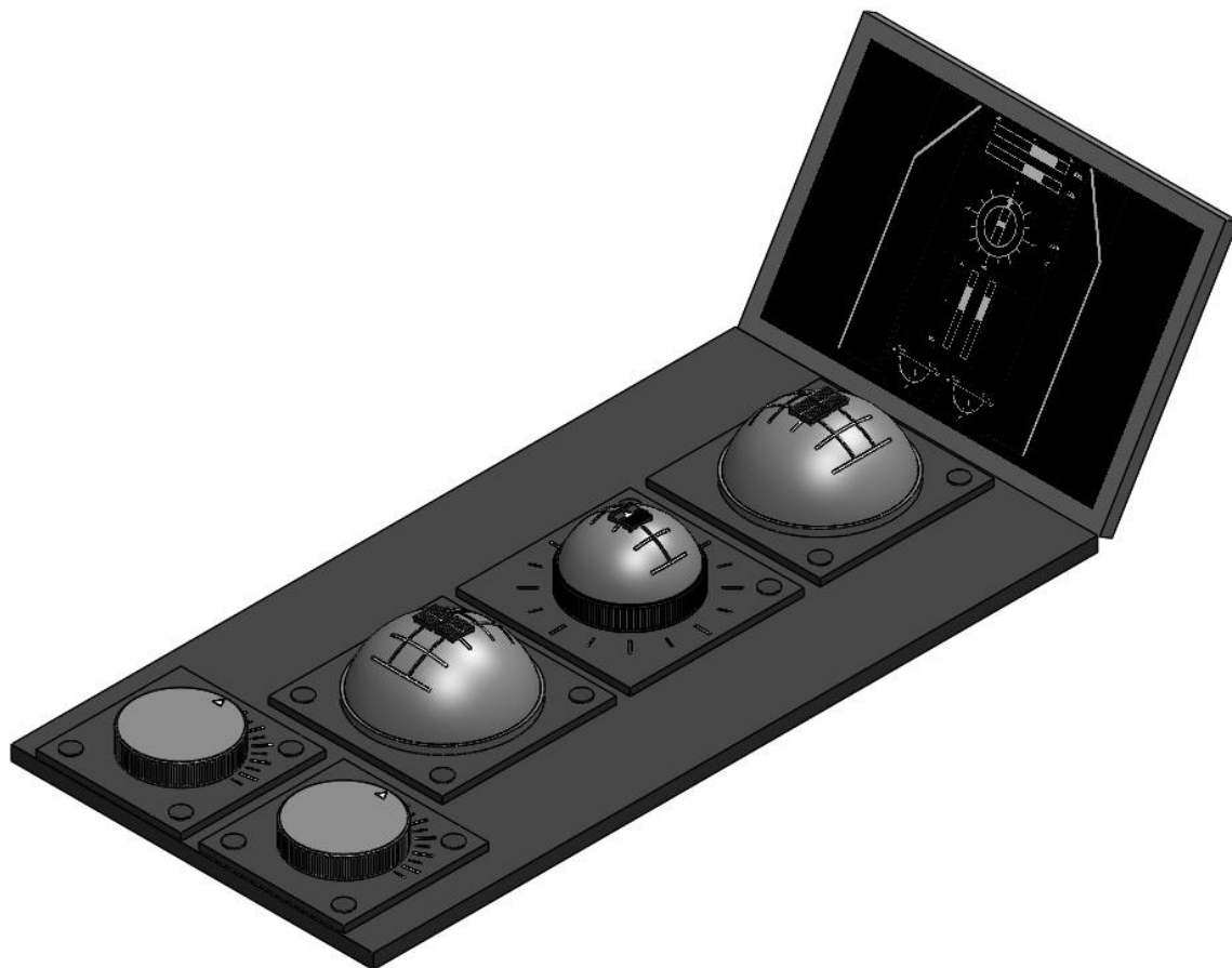
Figure 74: Setup consisting of two rudders, two speed levers, an azimuth lever and a corresponding display.
