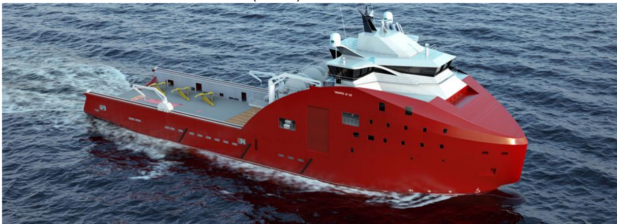
Figure 21: Anchor handling tug supply (AHTS). [48]
