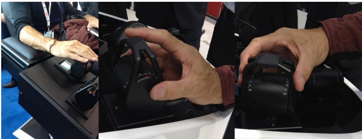
Figure 42: Lilaas L01 demonstrating the use of azimuth lever. (Own Photo)
