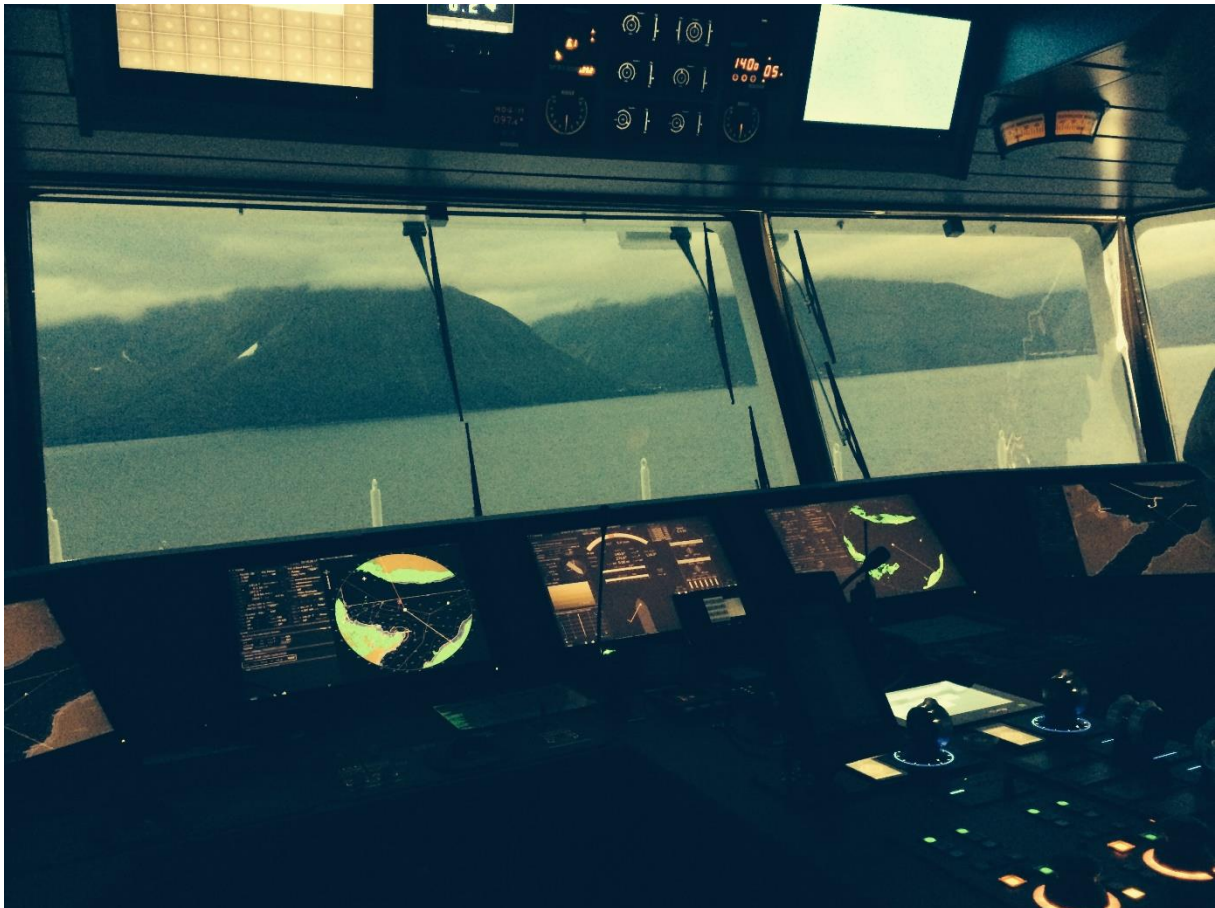
Figure 27: Dark bridge with illuminated equipment. [3, 4]
