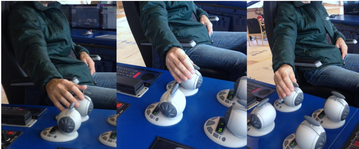
Figure 36: Demonstration of Helicon X3. A setup containing a split tunnel thruster lever and three azimuth levers. (Own photo)
