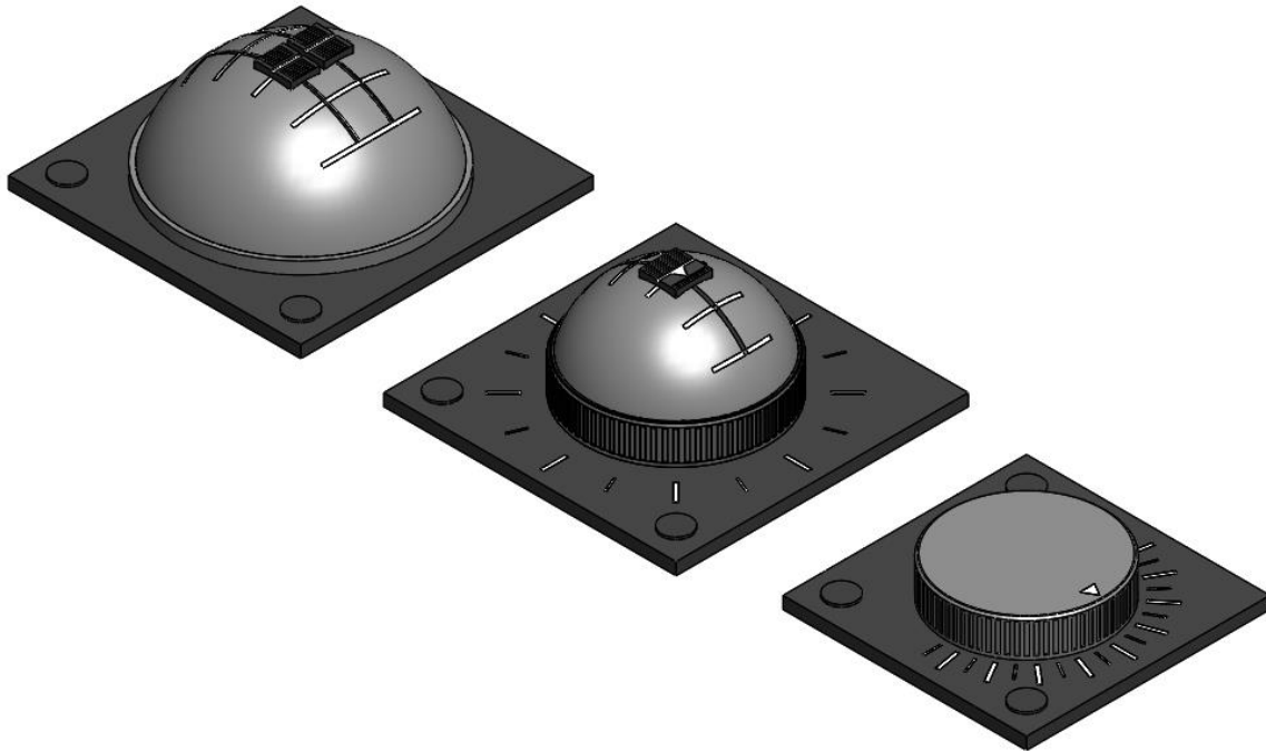
Figure 63: Final concept illustrating Speed lever, Azimuth lever and Rudder controller.
