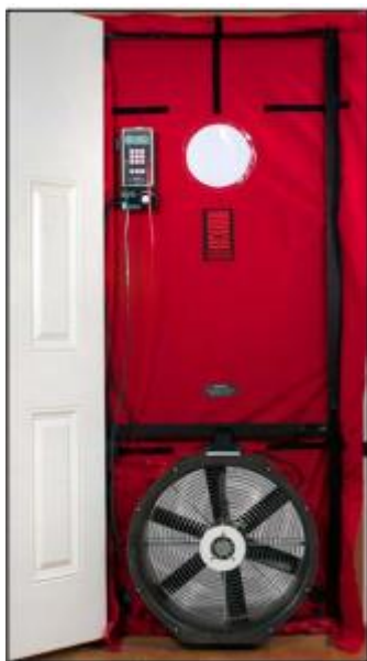
FIGUR 2-7: MINNEAPOLIS BLOWER DOOR-VIFTE (THE ENERGY CONSERVATORY).
