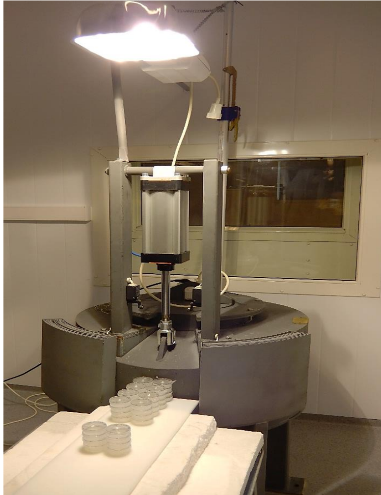
Figure 7. A. thaliana WT Ler and hy5 mutant seedlings in Petri dishes placed in front of a collimator and treated with gamma radiation from a ^{60}\text{Co} gamma source. Petri dishes were organized into two rows of columns (wild type vs hy5 mutant). The figure represents the second experiment, containing five columns, while the first experiment contained four columns.
