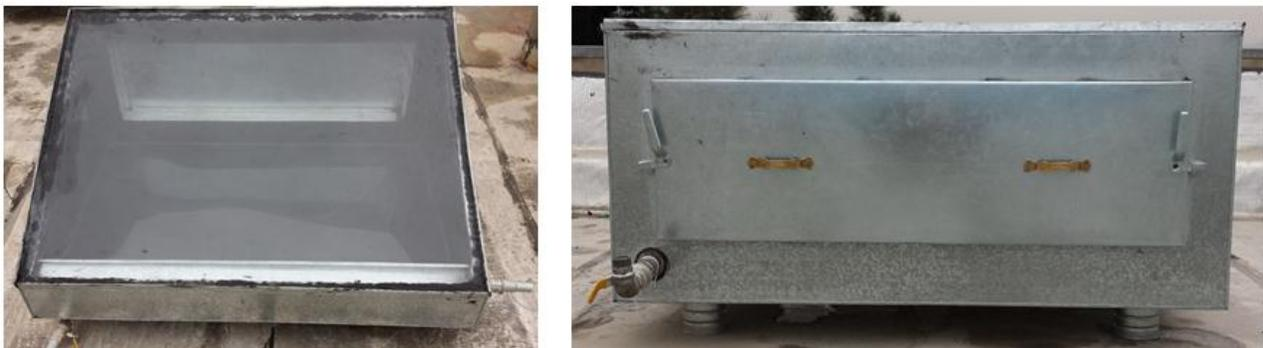
**Figure 33: Left: Front view of sloped glass cover and the flushing port can be seen down left. Down to the right comes the distillate output. Right: Back view with the inlet valve to the left and maintenance door in the middle.**
