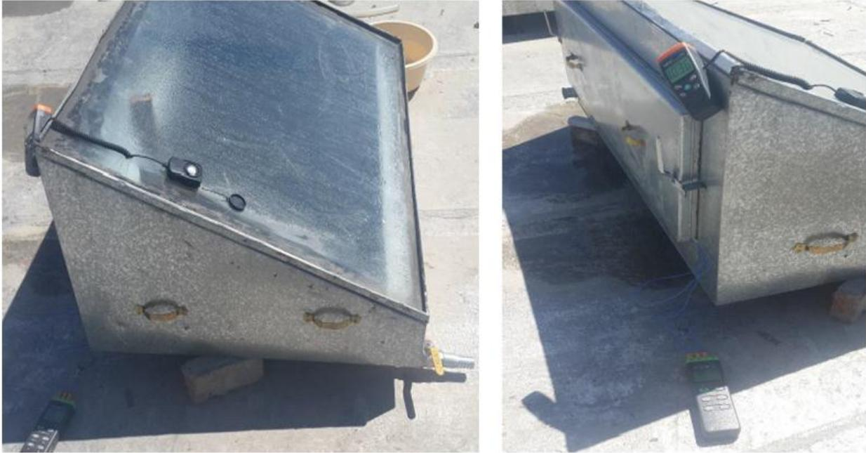
**Figure 39: Left: Testing of the solar still and measuring the incoming radiation on the glass surface. The glass surface is covered with condensed water. Right: The data logger on the ground is measuring water, vapor and glass temperature inside the still.**
