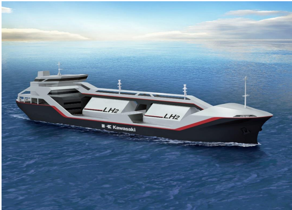
Figure 2.8: Prototype liquid hydrogen carrier ship. Source: (Kawasaki 2014)
