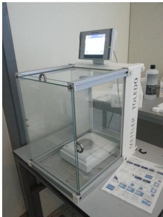
Figure 24: The Mettler Toledo Excellence Plus weight employed during research.
