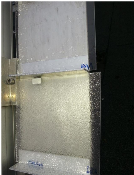
Figure 34: Two glass samples from the rooftop at IFE, Kjeller. The top sample is a normal glass sample, while the bottom sample is coated with the anti-soiling coating, TripleO.
