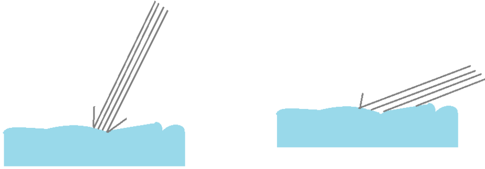
Figure 33: The incoming radiation is spread over a larger surface area at increasing angles of incidence.
