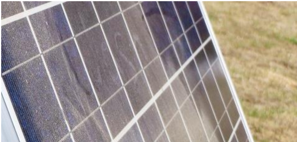
Figure 17: Soiling on PV-panels. Reprinted with permission © [21].
