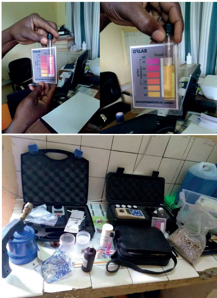
Figure 8. Water Quality sampling equipment at the Hygiene Service: Top left – a fluoride test on filtered water from my bottle, indicating between 0 and 0.5 mg/L of fluoride; Top right – a fluoride test on tap water indicating more than 3 mg/L of fluoride; Bottom – collection of assorted water quality testing equipment (Photos 19-08-19)
