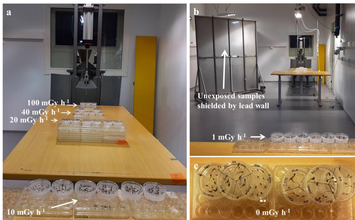
Figure 6. Gamma radiation exposure experiment set-up at the FIGARO low dose gamma irradiation facility. Petri dishes with six days old seedlings that were grown from seeds obtained from different areas in the Chernobyl region with background (CON), intermediate (INT) and high (TR22) levels of ionizing radiation (see Table 2) and the seedlings were exposed to gamma radiation with gamma dose rates ranging from 1 to 100 \text{mGy h}^{-1} for 144 h 7-12 days after sowing. a) The gamma radiation facility where the Petri dishes were positioned at different distances from the gamma radiation source to obtain the nominal dose rates. b) The gamma radiation experiment room showing the shielded lead wall where the unexposed samples were kept outside the radiation sector. c) The Petri dishes with seedlings that were placed behind the lead wall. All seedlings were in the same room under the same light and temperature conditions.
