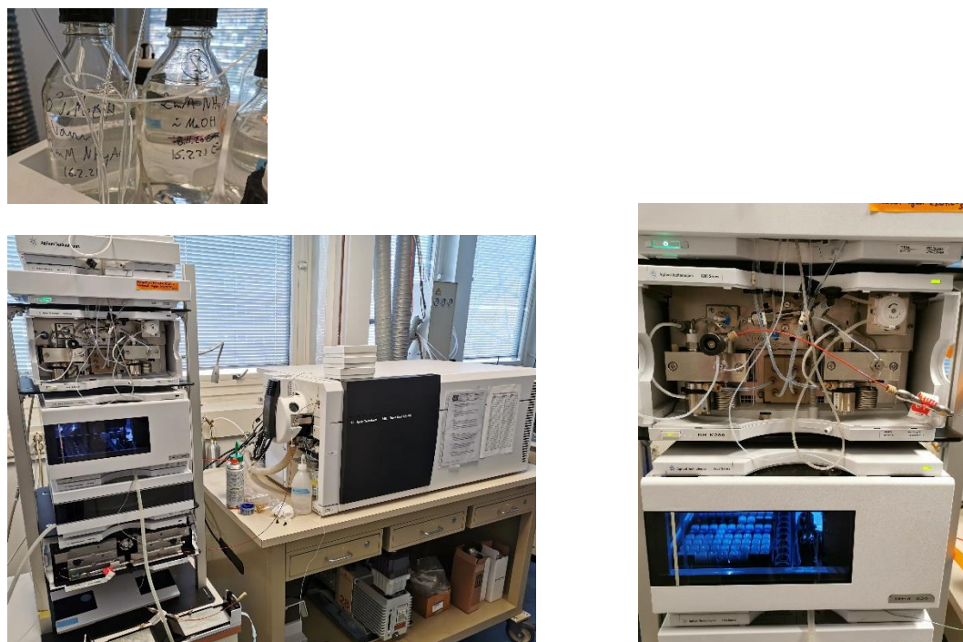
Figure 9 Agilent HPLC (left) system with MS detector (right). Bottles with mobile phases (over)
