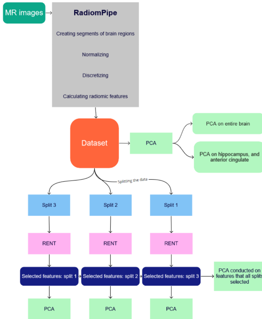
Figure 8: This figure displays a flowchart of the method applied in this thesis. The MR images were sent to RadiomPipe, which segmented the images. The image segments were further normalized and discretized, and radiomics features were calculated from these segments, resulting in a dataset. The dataset was split into a training and test set three times called split 1, split 2, and split3. RENT was applied to each one of these splits, where it selected a subset of the radiomics features. A PCA was conducted on the selected features from each of these splits. A PCA was also conducted on the features that were selected from all three splits. Further, a PCA was also conducted on the entire dataset and selected features corresponding to the brain regions, hippocampus, and anterior cingulate.
