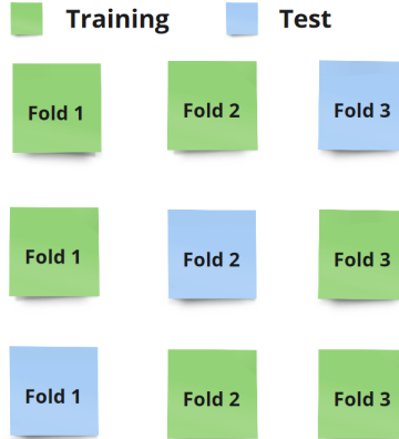
Figure 11: An overview of how the dataset was split into a training and validation set three times.
