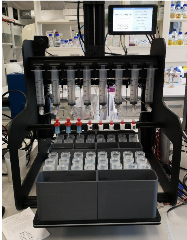
Figure 3.2. BigTrap used for Immobilized metal affinity chromatography (IMAC). Self-cleavable tag purification, a protocol for the robot made by Åsmund Røhr Kjendseth was used for the purification step. The Ni-NTA affinity chromatography columns are shown in the picture in blue and red. All fractions were collected in falcon tubes in front.
