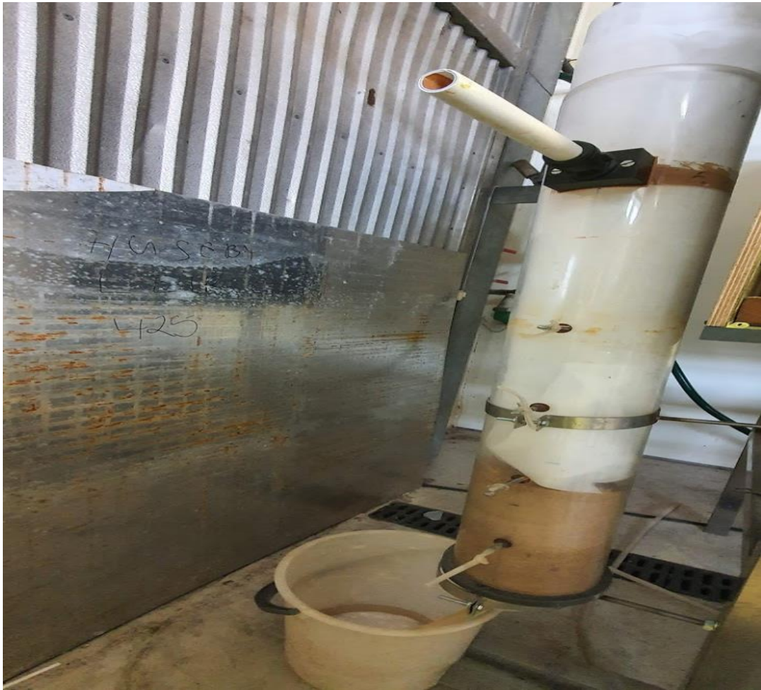
Figure 9: Filtration set-up used in sludge dewatering
