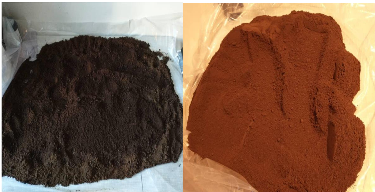
Figure 3: Wet SCG obtained from coffee shop (left) and the SCG after air drying (right)
