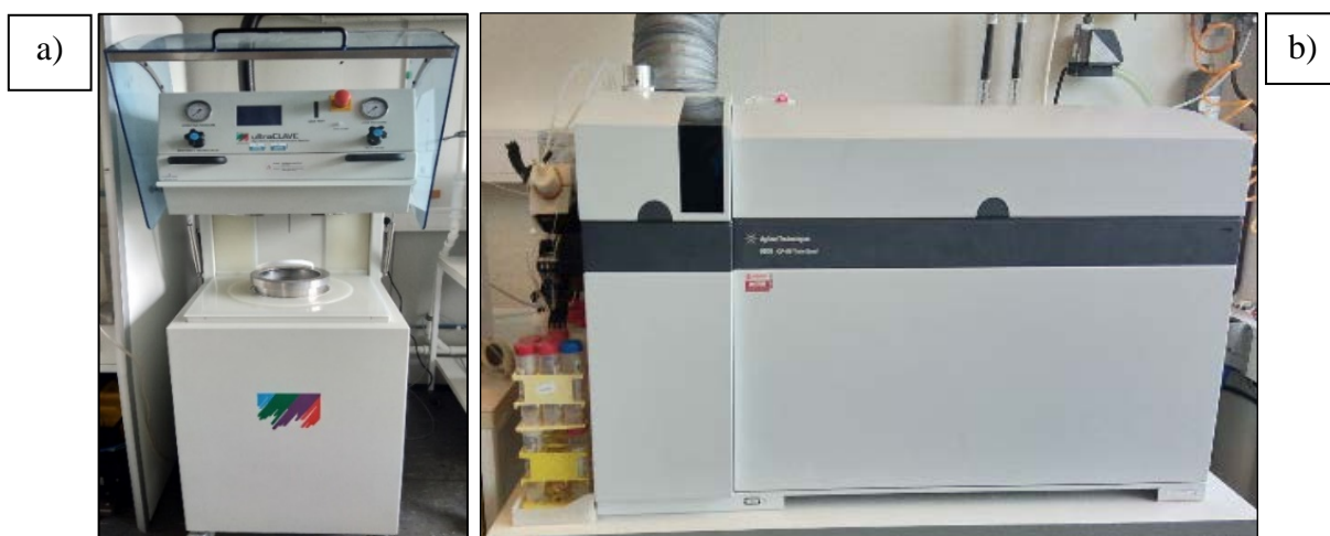
Figure 4.8 – Equipment for elemental analysis a) digestion set-up; b) ICP-QQQ-MS in He-KED (Ghent University, 2021)
