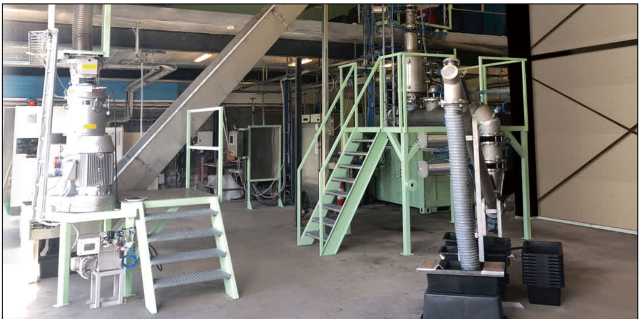
Figure 4.2 – Microwave-Assisted Pyrolysis system (MAP) (Scanship AS, 2019)
