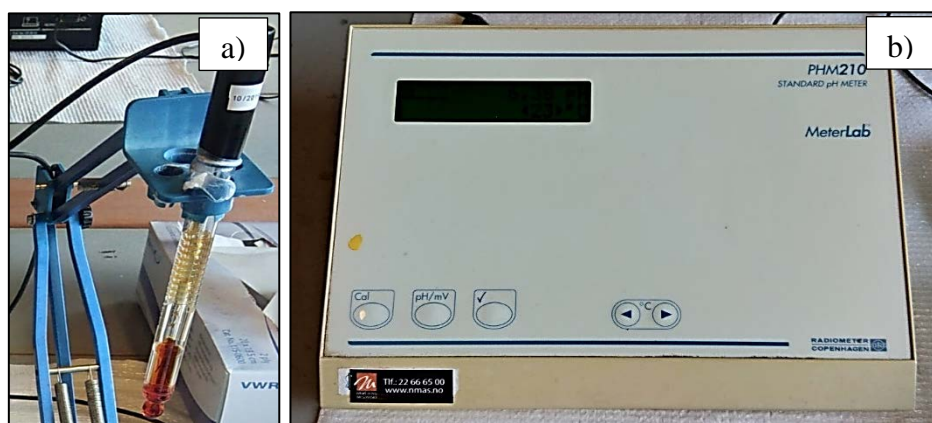
Figure B.4 Set-up for pH measurements: a) combined electrode; b) standard pH meter PHM210
