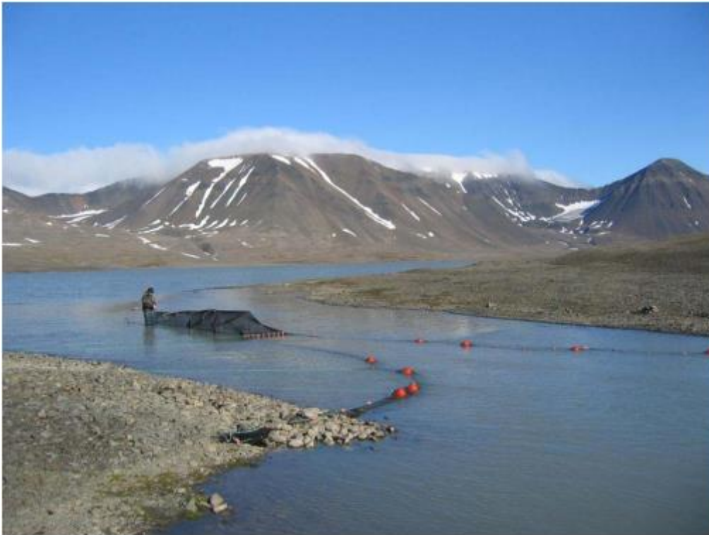
Figure 3: This picture shows how the migration trap looks. It consists of a ruse attached to two small meshed leading nets. The fish is trapped inside the fyke net, before it is taken to a tube for measurements and the surgical attachment of the transmitter. Photo: Martin A Svenning, NINA
