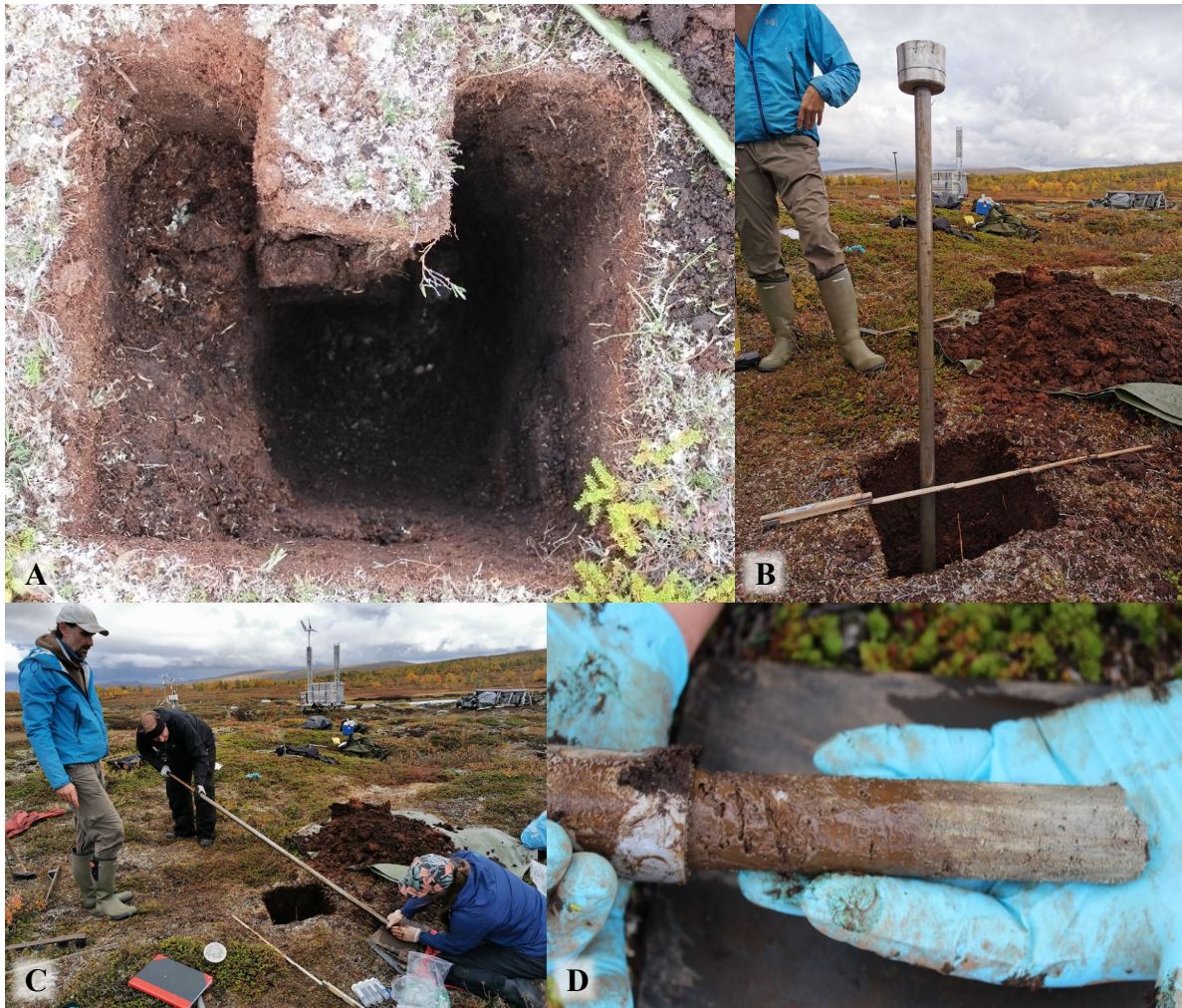
Figure 5. Stepwise sampling of palsa cores. (A) Removal of AL, leaving a protruding column for sampling undisturbed AL material. (B) Coring of permafrost using a metal tube. (C) Removing a sample from the cylinder by using a wooden broomstick. (D) Permafrost sample as it comes out from the cylinder. Shown is the bottom sample with transition to mineral soil.
