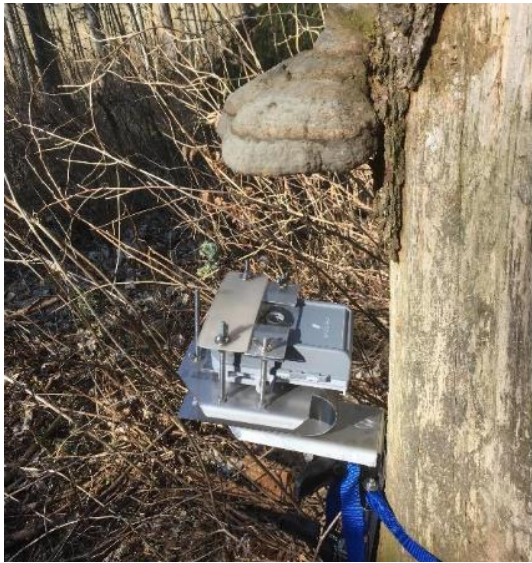
Figure 2. Setup showing the time-lapse camera attached beneath a fruiting body of F. pinicola using a custom mount. Photo: Tone Birkemoe
