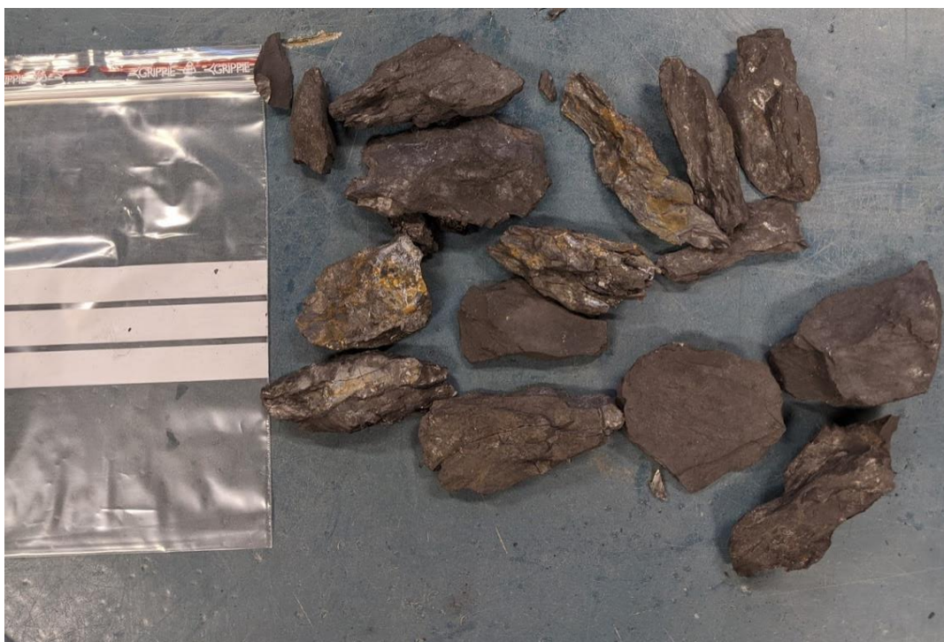
Figure 5: the stones from K34 that were crushed in the jaw crusher. Weathering can be seen from the yellow tint on some of the rocks. Photo: Johan Tryti, 11/11-2020.
