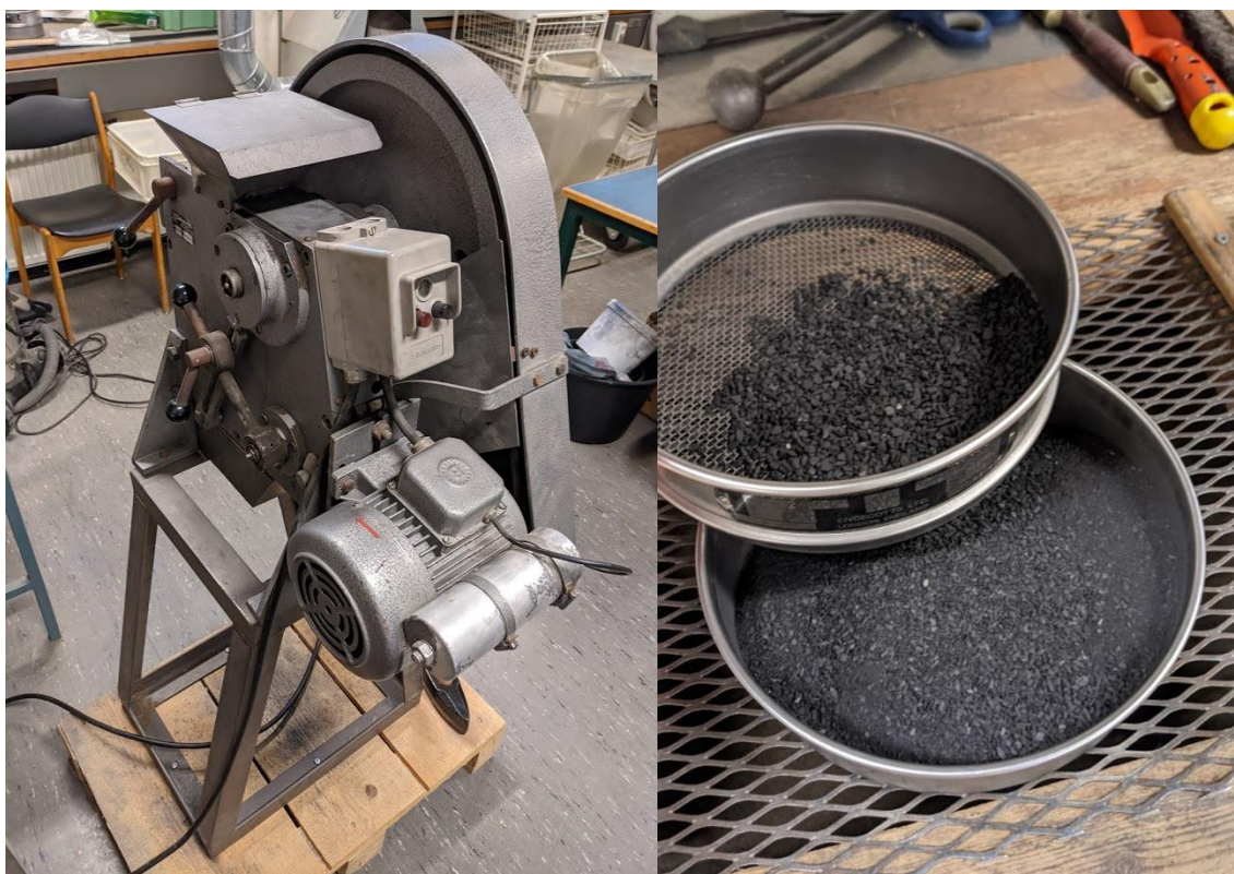
Figure 6: the jaw crusher used to crush the stone (left), and the resulting crushed alum shale (right). Photos: Johan Tryti, 11/11-2020.
