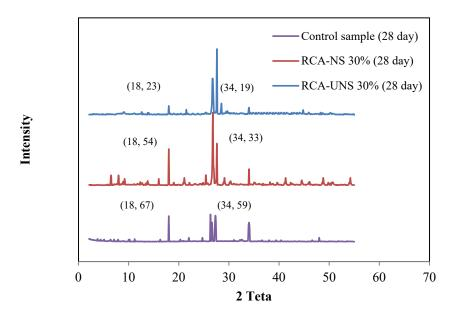
Figure 11. X-ray diffraction (XRD) of Control, RCA-NS 30%, and RCA-UNS 30% samples at 28 days.
