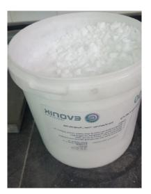
Figure 2. The nano-silica powder.
