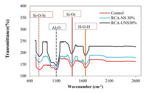
(RCA-UNS 30%) increased the Si–O–Si transmittance bands. The results of FT-IR graphs of samples were in agreement with compressive strength, SEM, and XRD results.
