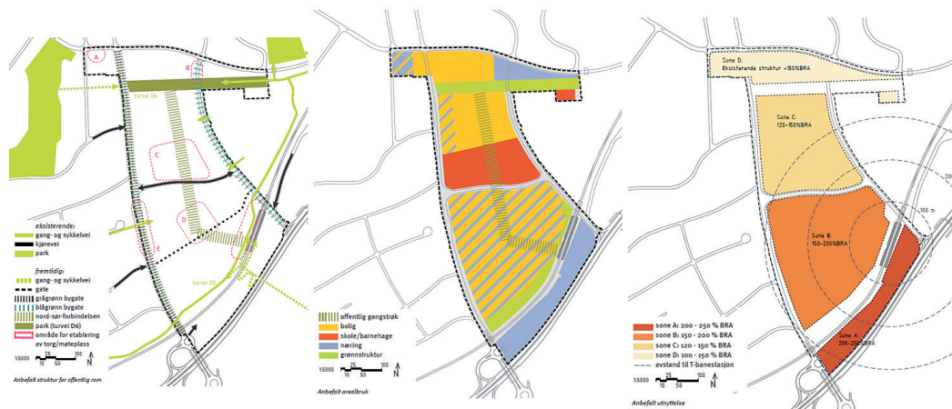
Fig. 1: Maps/plans from the VPOR for Vollebakk, Oslo. Left map shows main street network with squares and parks, middle map shows designated land use (yellow: residential, red: school/kindergarten, blue: business), right map shows accepted densities. The VPOR also consists of written descriptions that further elaborate on the criteria for development of Detailed Zoning plans.
